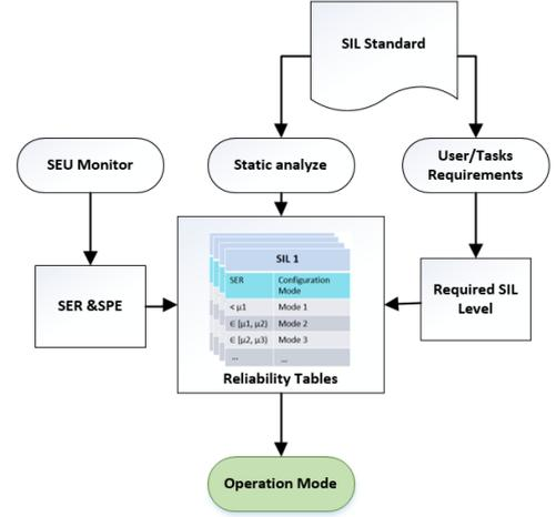
Fig. 2. Decision tree for determining the operation mode in the central analysis unit. The SIL standard is used here to quantify reliability requirements and establish an appropriate connection between the SERs from SEU sensor network with operation modes.
