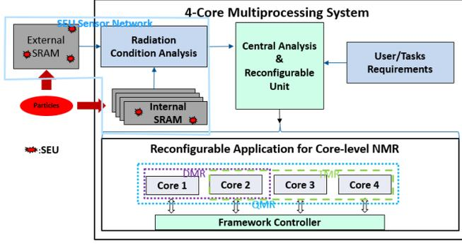
Fig. 1. Overview of the self-adaptive platform with 4-core multiprocessing system. The SEU sensor network can monitor the radiation particles and analyze the radiation environment. The appropriate core-level NMR operation mode can be decided according to the radiation environment and user/tasks requirements.
