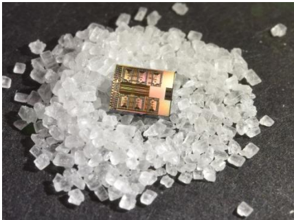
Monolithic integrated 28 Gbaud QPSK photonic receiver
