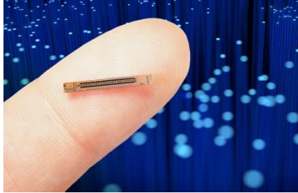
Monolithic integrated 32 Gbps silicon modulator with driver in 0.25 \mu m SiGe BiCMOS
