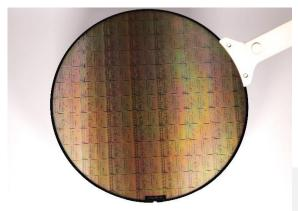
200 mm Si wafer featuring Graphene Photonic Integrated Circuits (PICs) fabricted in the BiCMOS pilot line at IHP within the framework of GATEPOST project ©IHP
