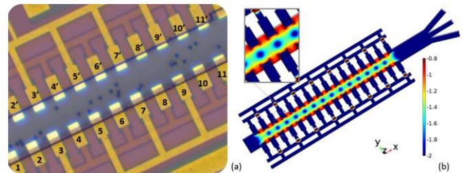
Fig. 1. Photograph of the proposed HF dielectrophoresis cytometer implemented on BiCMOS chip (a) and plot of the normalized electric field (log scale) once both side electrode pairs are biased with a 300MHz 3V magnitude signal.
