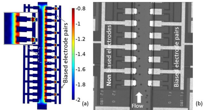
Fig. 2. Plot of the normalized electric field (log scale) once single side electrode pair's is biased with a 300MHz 3V magnitude signal (a), stacked images of a flowing single cell repelled by the E field gradient (b).
