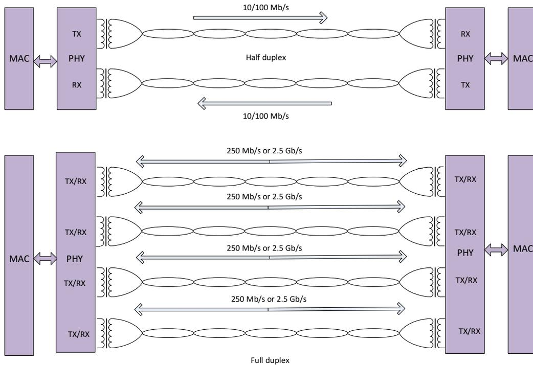
Figure 2 Transmission in 10BASE-T/100BASE-TX (top) and 1000BASE-T/10GBASE-T (bottom)
