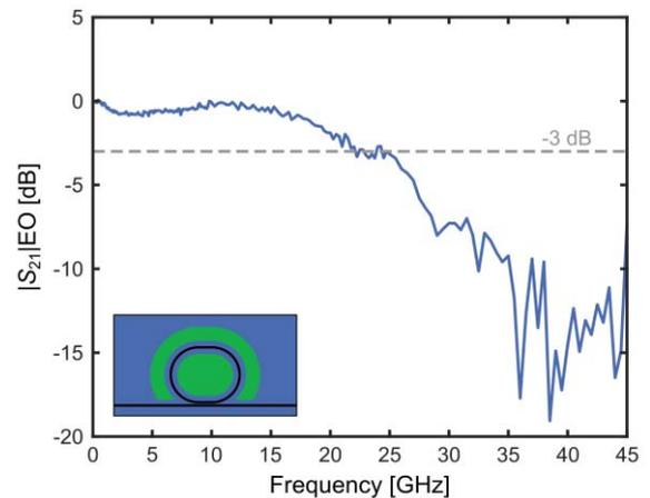
**Fig. 3:** Electro-optic bandwidth of a BaTiO<sub>3</sub> ring modulator. The flat response up to the photon lifetime limited cut-off is characteristic of the Pockels effect. The inset shows the schematic layout of the measured device.
