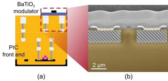
**Fig. 4:** (a) Integration scheme for monolithic integration of BaTiO<sub>3</sub>/Si devices on a Si photonics platform. (b) False-color SEM cross-section of BaTiO<sub>3</sub>/Si device fabricated on a Si PIC platform.
