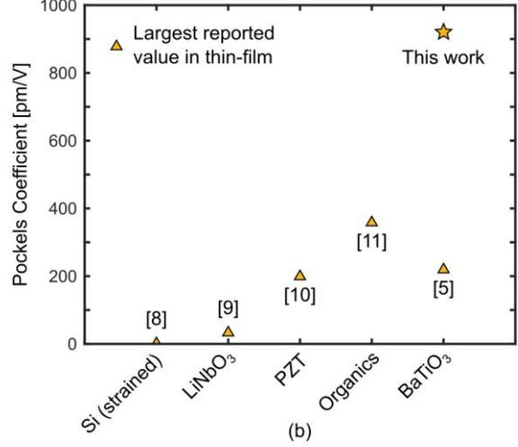
**Fig. 2:** (a) Electro-optic response of BaTiO<sub>3</sub>/Si devices as a function of device orientation for both TE and TM devices. An angle of 0° corresponds to devices with waveguides along the BaTiO<sub>3</sub> <100> direction. The large anisotropy is characteristic of the Pockels tensor of BaTiO<sub>3</sub>. (b) Comparison of the largest reported Pockels coefficients for thin-film materials.
