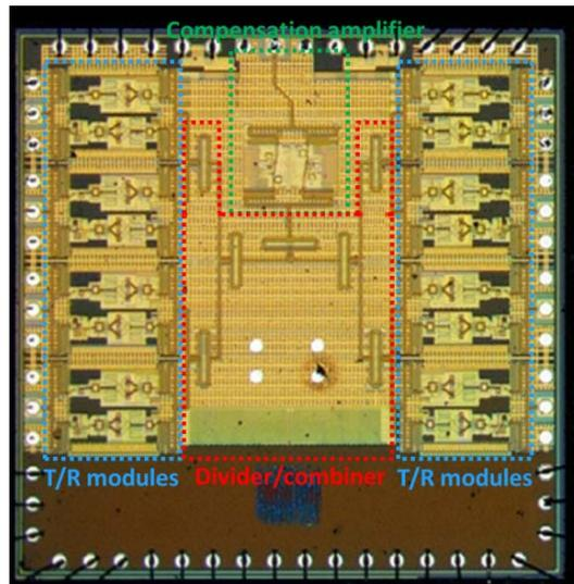
Fig. 4. Beamforming chip photomicrograph.
