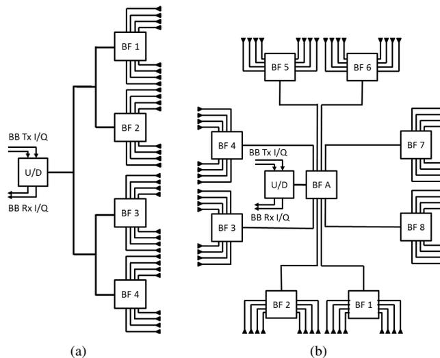
Fig. 1. Examples of modular beamforming systems: tree (a) and star (b).
