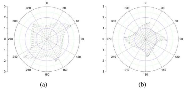
Fig. 8. Polar plot of the power gain in both Rx (a) and Tx (b) mode at a frequency of 62 GHz.
