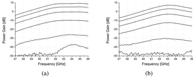
Fig. 7. Small-signal power gain varying the compensation amplifier gain in both Rx (a) and Tx (b) mode.
