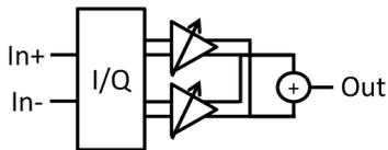
Fig. 3. Vector modulator architecture.
