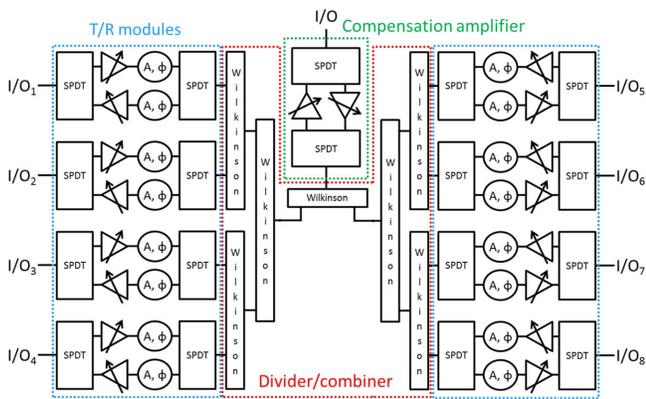
Fig. 2. Beamforming chip block diagram.
