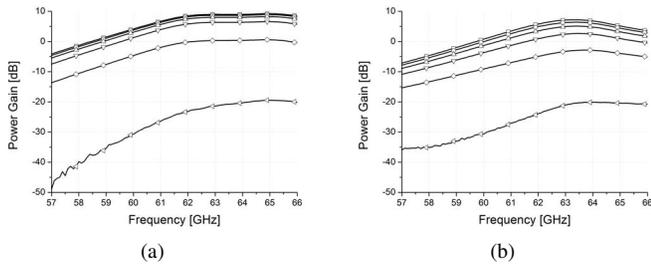
Fig. 6. Small-signal power gain sweeping LNA gain in Rx mode (a) and PA gain in Tx mode (b).
