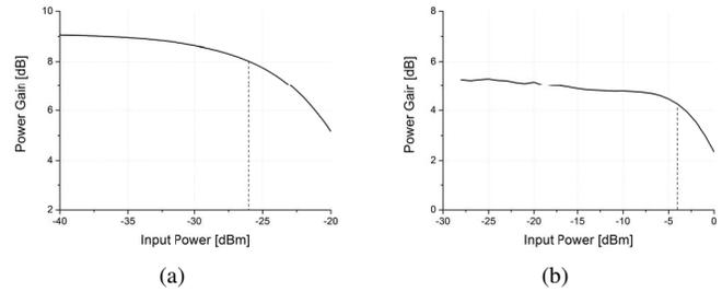
Fig. 9. Power gain versus input power in both Rx (a) and Tx (b) mode, measured at 63 GHz and 62 GHz respectively.
