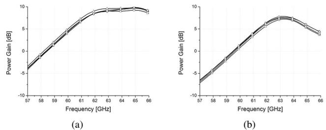
Fig. 5. Small-signal power gain along 4 of the 8 channels in both Rx (a) and Tx (b) mode.
