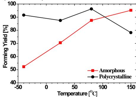
Fig.3: Forming Yield as function of temperature in Amorphous and Polycrystalline arrays.
