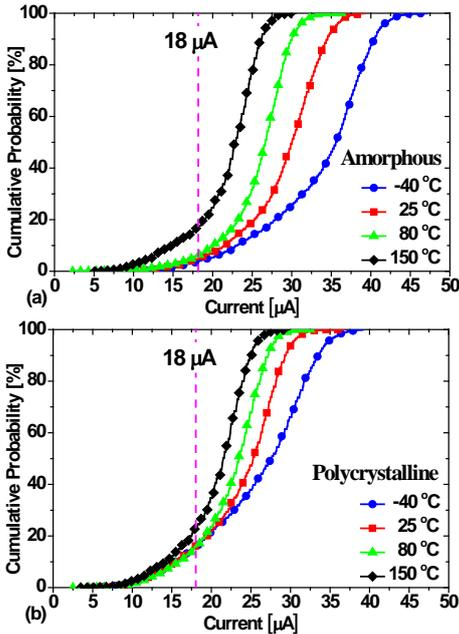
Fig.8: Current cumulative probabilities at the end of ISPVA forming operation, respectively, in A-arrays (a) and P-arrays (b).
