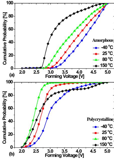
Fig.5: Forming voltage cumulative probabilities at the selected temperature values in A-arrays (a) and P-arrays (b).
