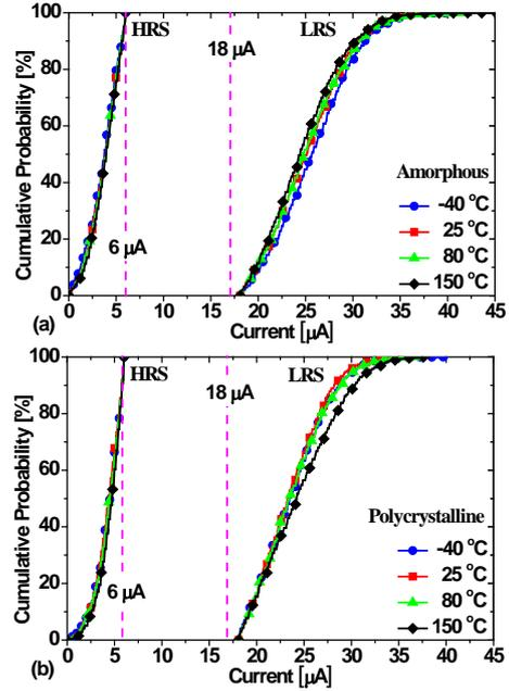
Fig.6: HRS and LRS current cumulative probabilities after reset and set operations, respectively, in A-array (a) and P-array (b).
