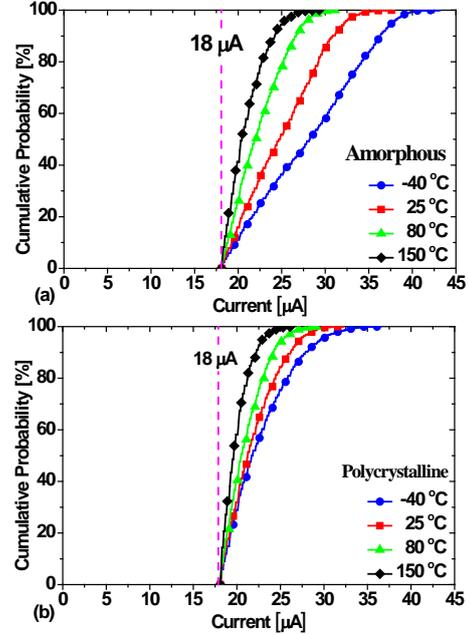
Fig.4: Current cumulative probabilities just after forming at the selected temperature values in A-arrays (a) and P-arrays (b).
