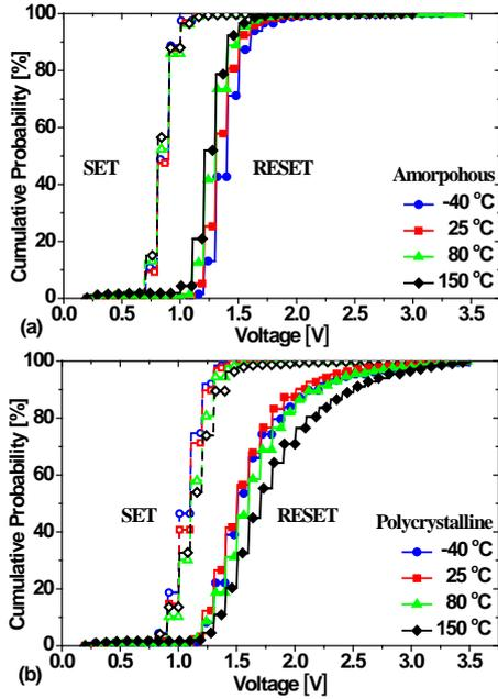
Fig.7: Reset and set voltage cumulative probabilities at the selected temperature, respectively, in A-arrays (a) and P-arrays (b).
