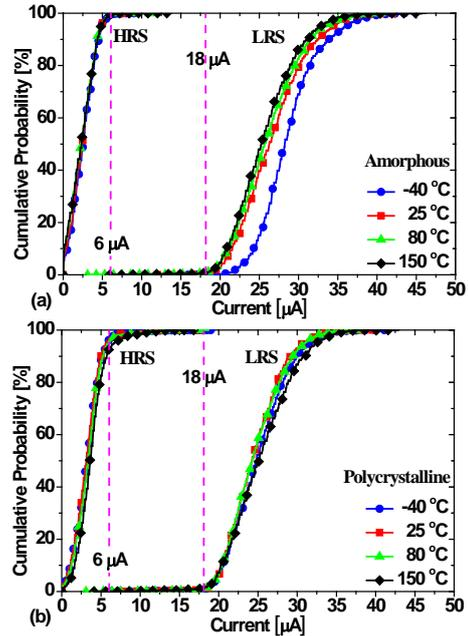
Fig.9: HRS and LRS current cumulative probabilities at the end of ISPVA reset and set operation, respectively, in A-arrays (a) and P-arrays (b).
