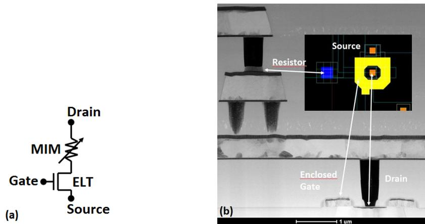
**Figure 1.** Circuit schematics (a) and TEM cross-sectional image of 1T-1R architecture with an ELT transistor and a 0.7 x 0.7 μm<sup>2</sup> MIM cell (b).
