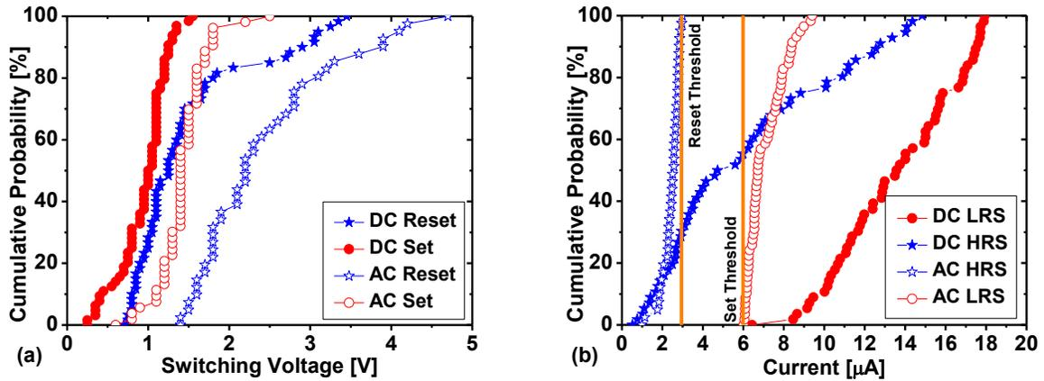
**Figure 4.** Cumulative distributions of the reset/set voltages (a) and HRS/LRS currents (b) in DC and AC mode.
