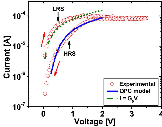
**Figure 6.** Reset I-V characteristics measured in DC mode. The solid line represents the adaption of the QPC model detailed by equation 1.
