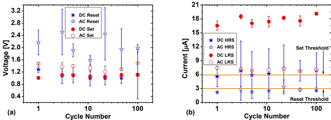
**Figure 5.** Average and dispersion values of reset/set voltages (a) and of HRS/LRS currents (b), received by applying DC and AC modes as function of cycling.
