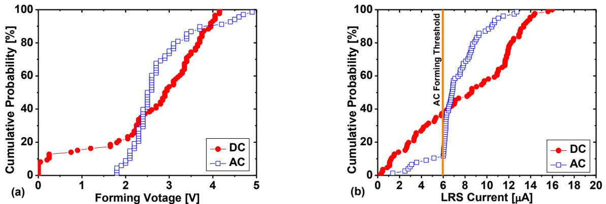
**Figure 3.** Cumulative distributions of forming voltages (a) and LRS currents (b) in both modes.
