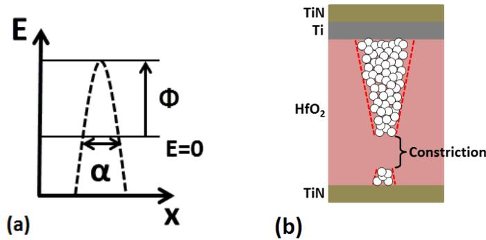
**Figure 2.** Schematic illustration of QPC barrier parameters (a) and of the conductive filament shape after reset (HRS) (b).
