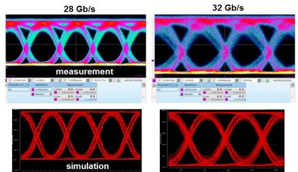
Fig. 5. Measured and simulated EO eye-diagrams at 28 and 32 Gb/s when  $V_{bias}$  is equal to 1 V.
