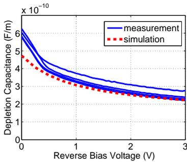
Fig. 3. Phase shifter depletion capacitance change with reverse bias voltage.
