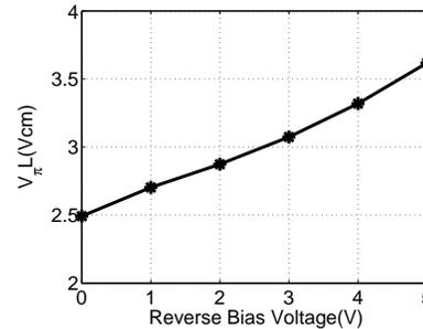
Fig. 2. Phase shifter inverse efficiency  $V_{\pi} \cdot L$  extracted from measurements.
