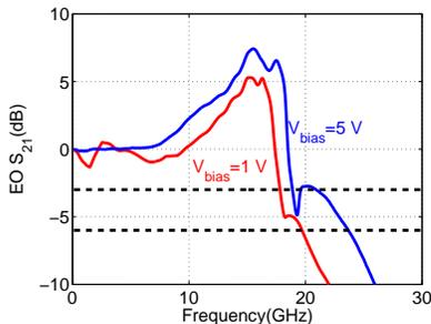
Fig. 4. Normalized measured EO  $S_{21}$  with frequency when  $V_{bias}$  is equal to 1 and 5 V.
