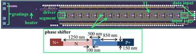
Fig. 1. Microphotograph of the monolithically integrated Si SE-MZM.
