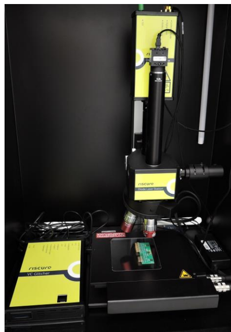
Fig. 1. Riscure Diode Laser Station as a part of the laboratory equipment at the IHP:
