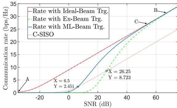
Figure 4. Communication rate curves for Exhaustive and Hierarchical beam searches;  $N_{TX} = 64$   $N_{RX} = 8$   $k = 3$
