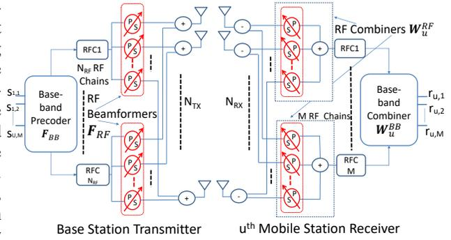
Figure 1. System model: BS serving  $U$  MSs with transmission of  $M$  streams per MS [15].
