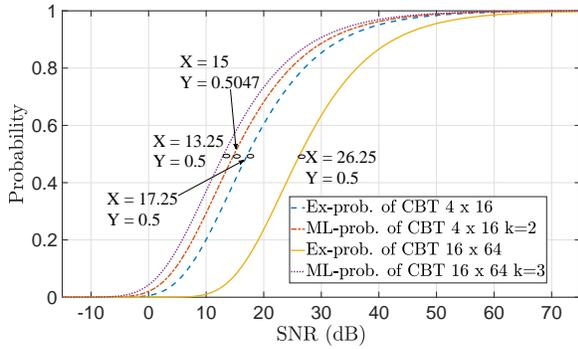
Figure 3. Probability curves for correct beam selections for Exhaustive and Multi-level beam searches
