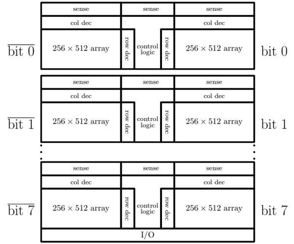
Fig. 2. Block arrangement of the 1Mbit structure.
