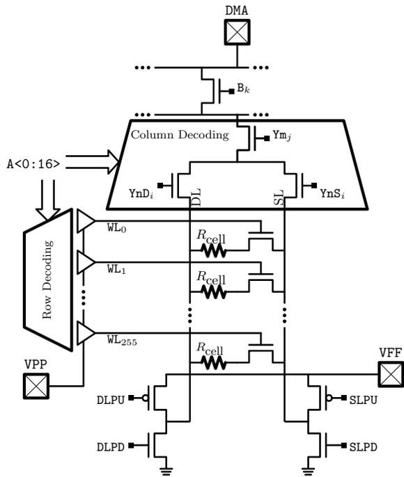
Fig. 4. DMA architecture
