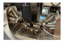
Electromechanical RF-MEMS Characterization based on Laser-Doppler Vibrometry
