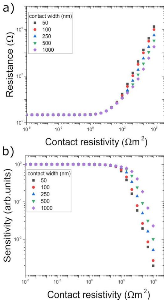
Fig. 3. Typical quantities accessible from the simulations: The device resistance (a) and the expected sensitivity (b). Fixed parameters used: electrode spacing 500 nm, specific resistivity 10<sup>9</sup> Ω cm.
