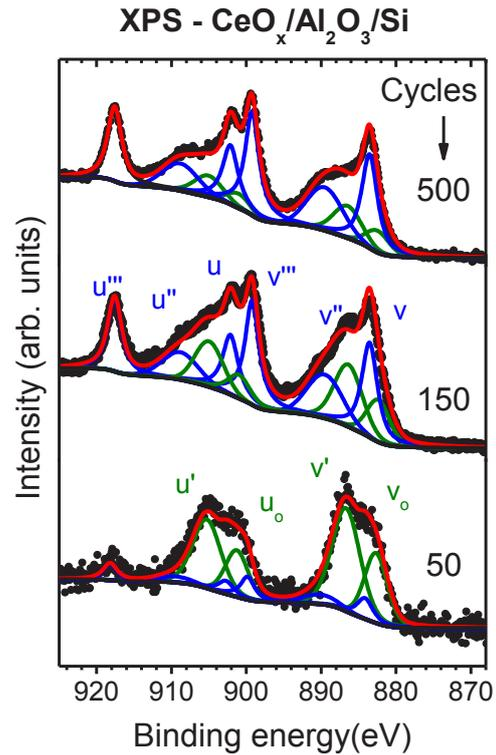
Fig. 2. In-situ XPS Ce 3d core level spectra taken from ALD ceria films of various thicknesses.
