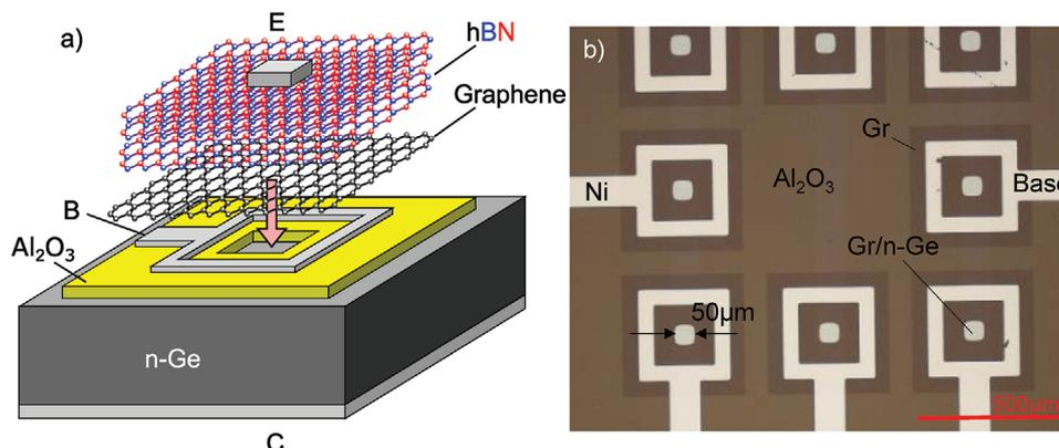
**Figure 1.** a) 3D representation of the hot electron transistor with a multilayer hexagonal boron nitride (hBN) emitter-base (E/B) insulator, a monolayer graphene base (B), and an n-Ge collector (C) semiconductor. b) Top view of the hot electron transistor after lithography and subsequent wet transfer of hBN.
