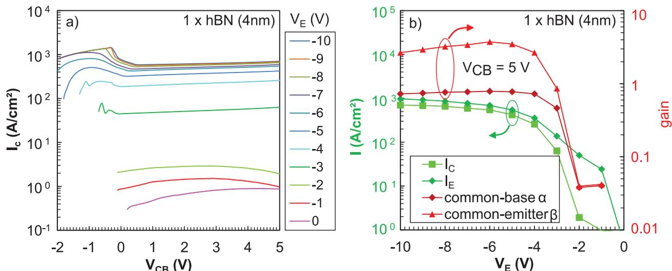
**Figure 5.** a) Common-base output characteristics of the hBN/Gr/n-Ge hot electron transistor with the emitter voltage as a parameter. b) Emitter current, collector current, and gain of the hot electron transistor as a function of the emitter voltage.
