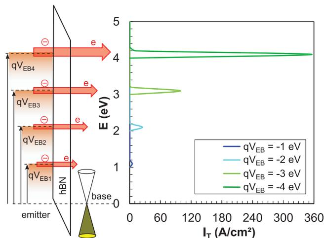
**Figure 6.** Energetic distribution of the calculated emitter-base tunneling current density  $I_T$  through 4 nm hBN with the parameter  $qV_{EB}$ .
