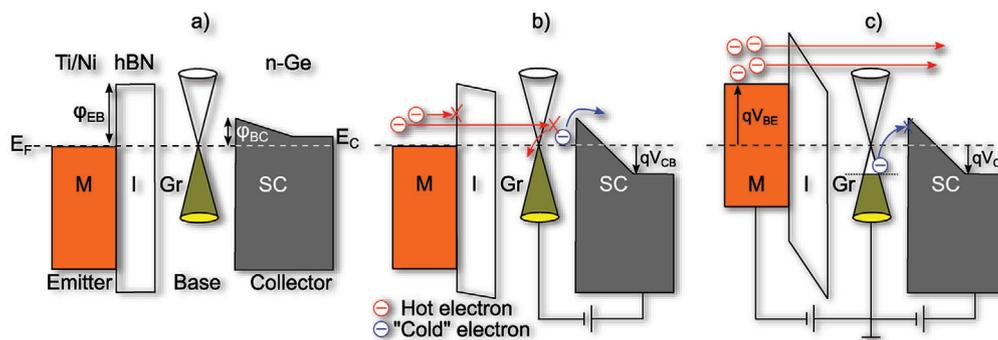
**Figure 2.** Simplified band scheme of the metal (M), insulator (I), graphene (Gr), semiconductor (SC) hot electron transistor in a) thermal equilibrium, b) OFF-state, and c) ON-state.
