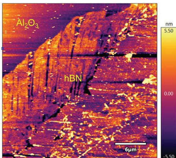
**Figure 3.** AFM image of wet transferred hexagonal boron nitride (hBN) on aluminum oxide ( $\text{Al}_2\text{O}_3$ ).
