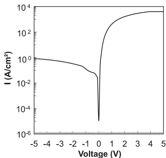
**Figure 4.** IV characteristics of the base-collector Schottky diode representing the graphene/n-Ge junction.
