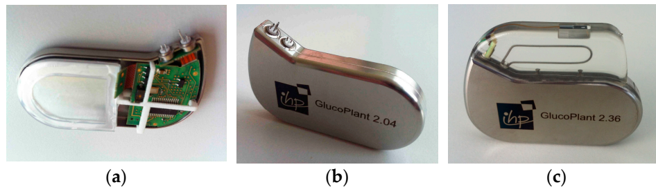
Figure 5. Biosensor implant (a) prior to and (b) after closing the Ti shucks by laser welding; (c) Fully implantable system including header with antenna and sensor probe (59 mm × 45 mm × 8 mm).
