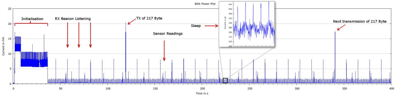
Figure 2. Power plot of a BSN with a full application cycle of 221.48 s during normal operation
