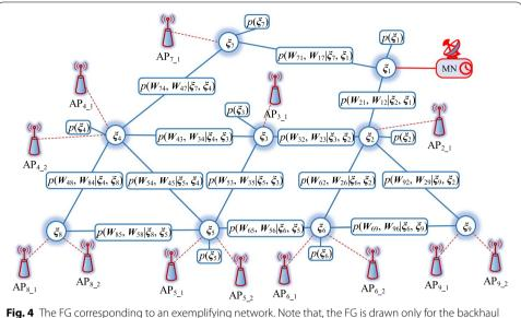
**Fig. 4** The FG corresponding to an exemplifying network. Note that, the FG is drawn only for the backhaul network to avoid unnecessary complexity. To draw the FG of the whole network, one can simply consider APs as variable nodes connected to their corresponding backhaul nodes via factor nodes
