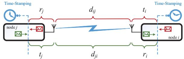
Fig. 2. Delay decomposition.
