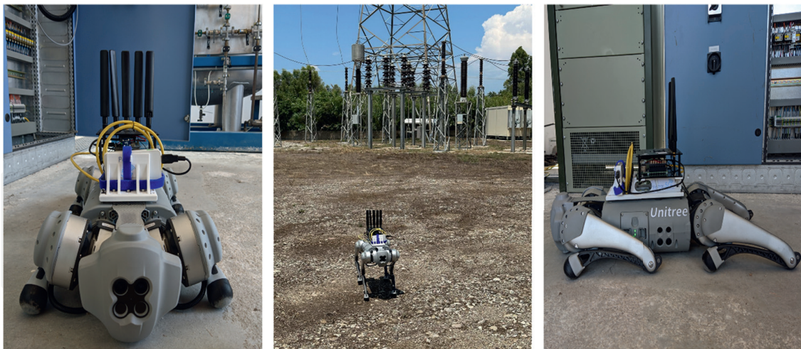
Figure 5. Facilities security: 5G-enabled mobile surveillance robot in action.
