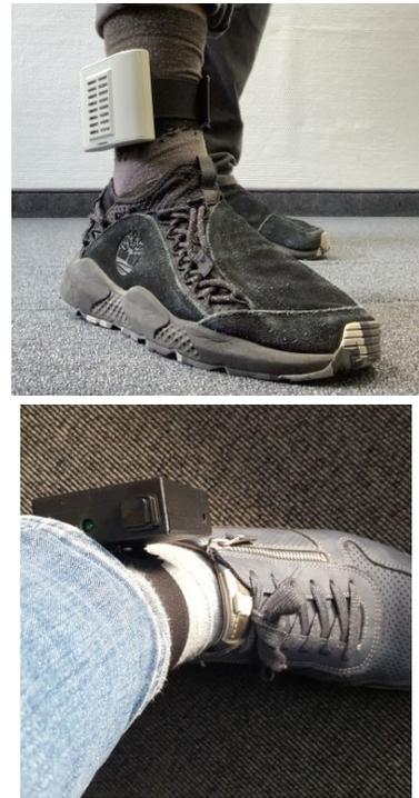
Figure 1: Google coral mounted on shank (upper). The cueing device, lower image, receives the trigger command whenever the FOG detected the ML model on Google Coral.
