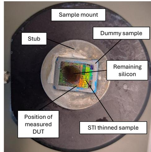
Figure 4: Overview image of the STI thinned sample, sample stub holder and sample mount. Picture taken before sample release.
