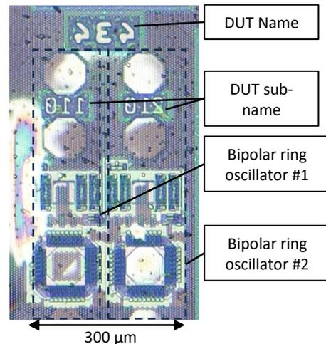
Figure 5: Full removal of the backside silicon allows to directly look at the device level, using an optical microscope.
