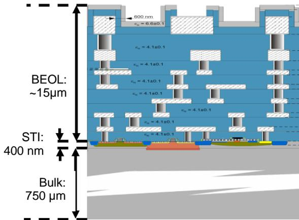
Figure 3: Schematic IC cross section of the IHP BiCMOS process [7].
