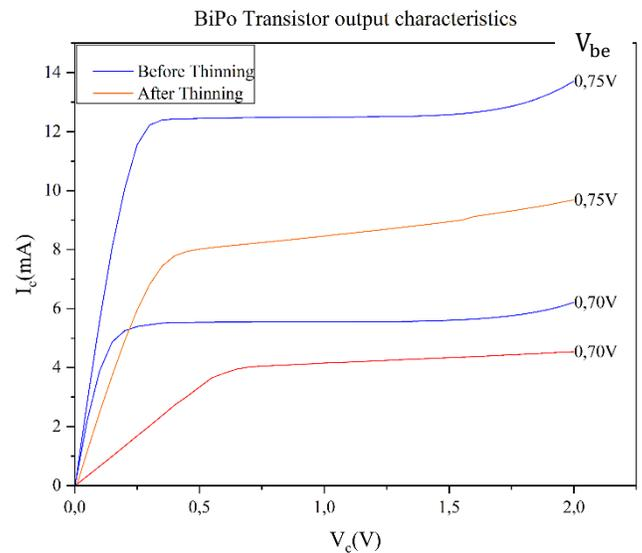
Figure 8: Output characteristics of a single bipolar transistor before thinning and after thinning to STI level.
