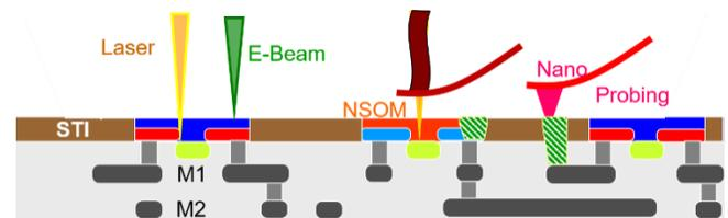
Figure 1: High resolution fault isolation techniques [4]
