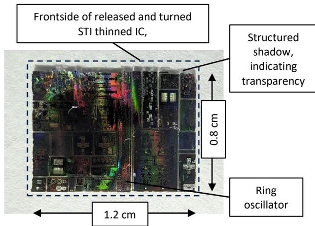
Figure 6: Front side image of an STI chip that has been release and placed on a filter paper. Total remaining thickness of the shown chip is approximately  $15\ \mu\text{m}$ .
