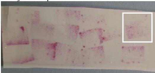
Figure 2: Used Fujifilm's Prescale; pressure marks for adjustment of parallelism between sample and pad. White frame shows optimum
