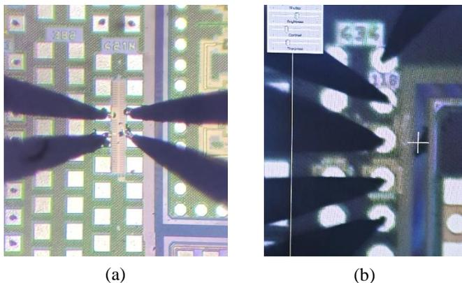
Figure 7: Needle probed test structures after STI thinning: (a) single transistors; (b) ring oscillators.
