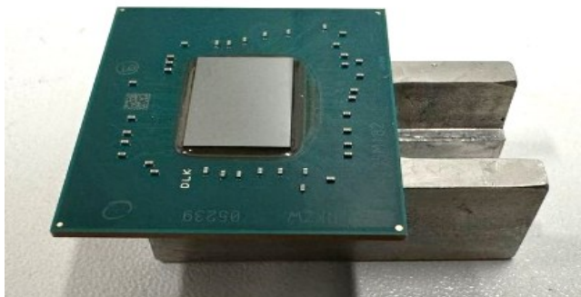
Figure 5: Flip-Chip mounted sub 50nm device mounted; carrier PCB mounted on a customised sample holder for the Allied Multiprep; Protective blocking capacitors not yet removed.
