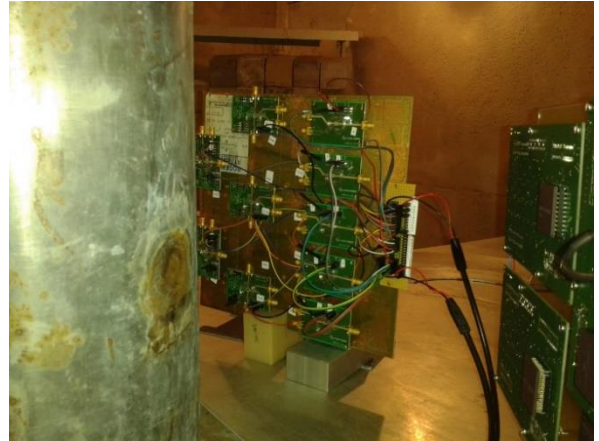
Figure 16: TID radiation set up of PLL and TRX boards at HZB
