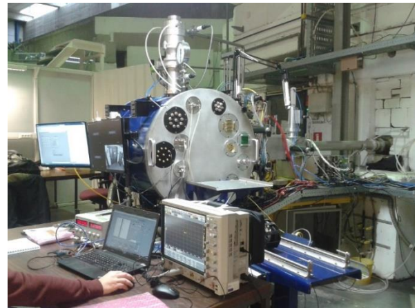
Figure 22: SEE measurement environment
