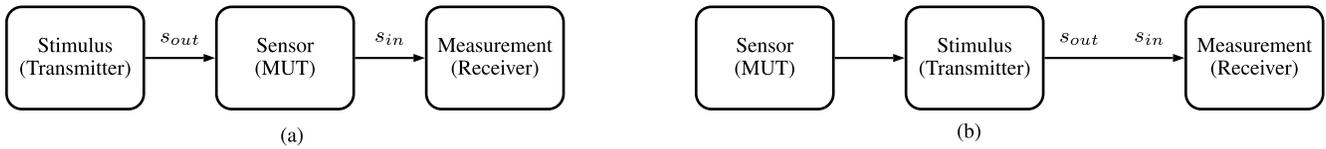
Fig. 1. Block diagram of (a) transmission-based analyzer and (b) analyzer based on the readout of a stimulus manipulated by a sensor element.
