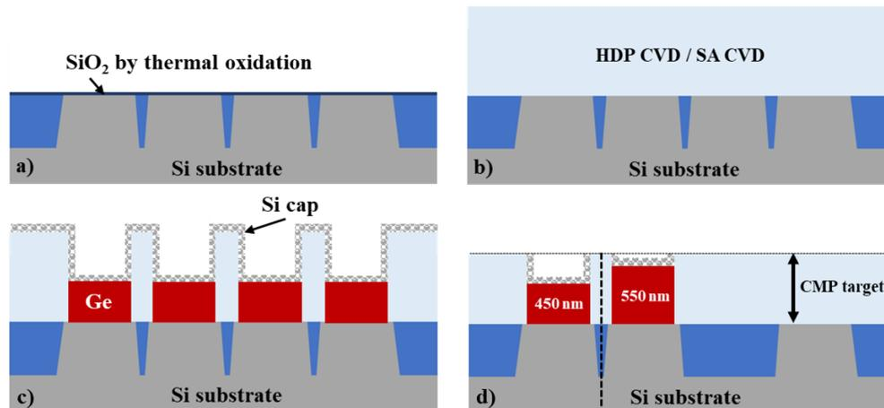
**Fig. 2.** Schematic description of the realization of the Ge stripes for the photodetector: (a) Thermal oxidation after the STI module; (b)  $\text{SiO}_2$  deposition by various CVD procedure; (c) Ge epitaxy selective to  $\text{SiO}_2$  followed by a differential epitaxy of a Si cap; (d) Removal of the Si cap on the  $\text{SiO}_2$  surface by CMP
