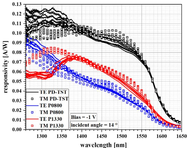
**Fig. 14.** Responsivity measurement in dependence on the wavelength of PD-TST, P0800 and P1330 under illumination with TE and TM polarized using an incident angle of  $14^\circ$  and a bias of  $-1$  V
