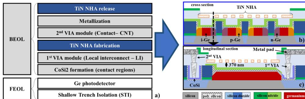
**Fig. 3.** (a) Schematic description of the technology process for the cointegration of Ge photodetectors and TiN NHAs as well as (b) a schematic cross section and (c) longitudinal section (at marked point in Fig. 3(b)) of the device
