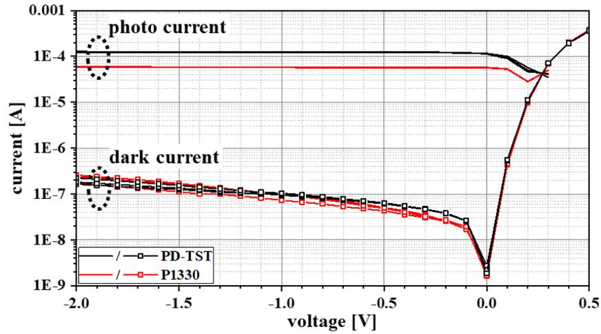
**Fig. 12.** Dark current and photo current of PD-TST and P1330 measured via top illumination with TE polarized light at  $\lambda = 1310$  nm using an incident angle of  $14^\circ$  and an optical power at fiber end of 1 mW
