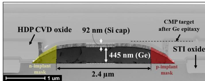
**Fig. 6.** TEM inspection of the cross section of one stripe of PD-TST
