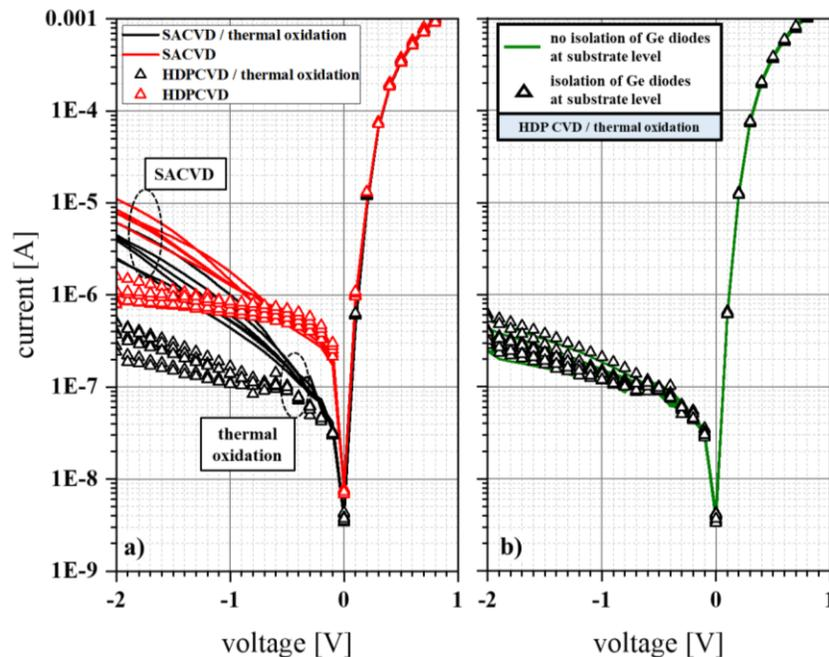
**Fig. 5.** IV characteristics of several PD-TST devices (a) for different process variations and (b) different design concepts ( $t_{\text{Ge}} = 450 \text{ nm}$ )
