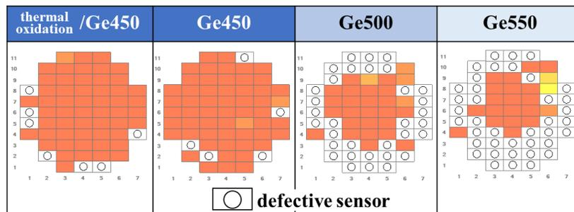
**Fig. 7.** Wafer distribution of defective P0800 devices for various process variations
