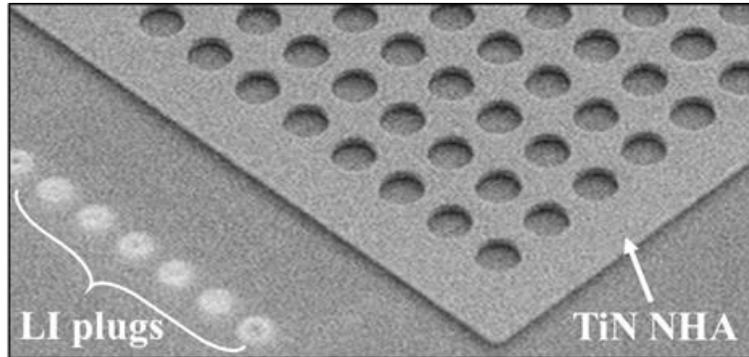
**Fig. 8.** SEM inspection after the fabrication of the TiN NHA in the BEOL
