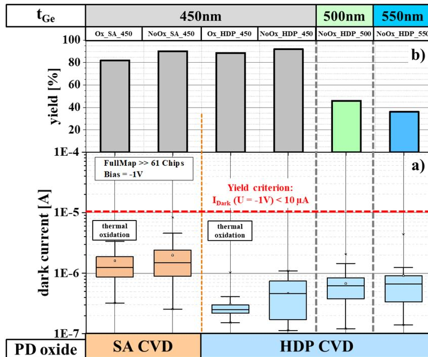
**Fig. 4.** (a) Full wafer measurement of dark current at a bias of  $-1$  V and (b) analysis of the yield for various process variations of P0800; yield criterion:  $I_{\text{Dark}}(U = -1 \text{ V}) < 10 \mu\text{A}$
