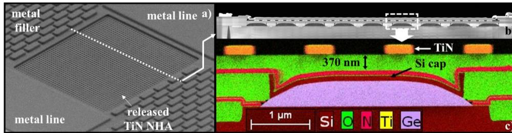
**Fig. 10.** a) SEM inspection of the released TiN NHA; b) TEM images of the cross section of P1330; c) EDX analysis of one Ge stripe of P1330
