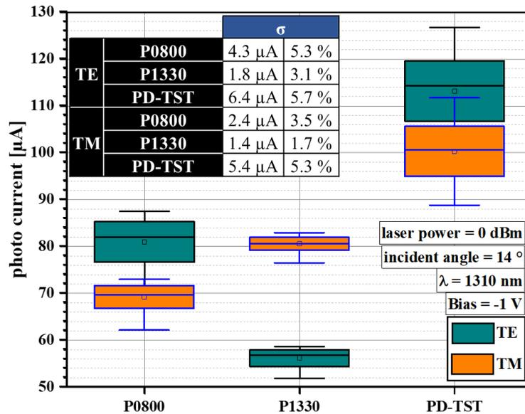
**Fig. 13.** Full wafer measurement of the photo current at a bias of  $-1$  V measured via top illumination with TE/TM polarized light at  $\lambda = 1310$  nm using an incident angle of  $14^\circ$  and a laser power at fiber end of 1 mW. For P1330 our results show not only a marked polarization dependence of photocurrents compared to P0800 and PD-TST but also an excellent homogeneity over the full area of the wafer.
