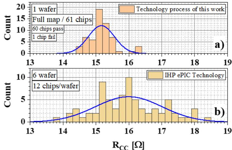
**Fig. 9.** Histograms of the contact resistance (a) for the technology process of this work and (b) for the IHP ePIC technology
