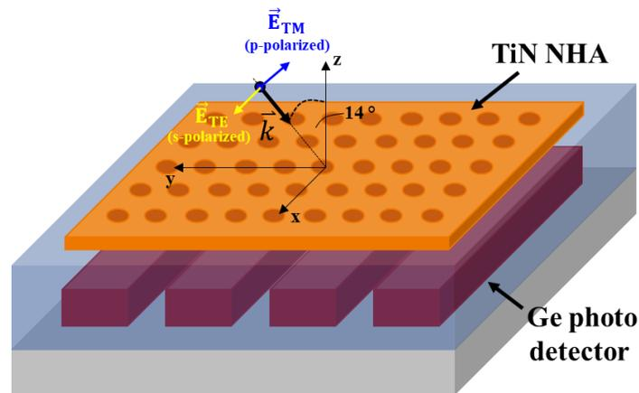
**Fig. 11.** Schematic of the device top illuminated with TE/TM polarized light under an incident angle of 14°
