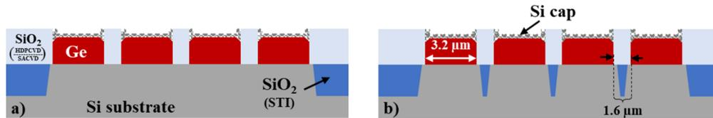
**Fig. 1.** Schematic of Ge photodetector stripes (a) without and (b) with additional isolation at Si substrate level
