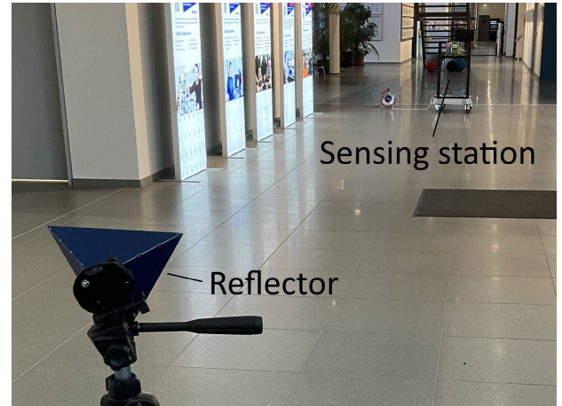
FIGURE 10. Measurement setup with up to 60 m distance (currently 10 m) between the JCAS transceiver and a RADAR corner reflector in an entrance hall.
