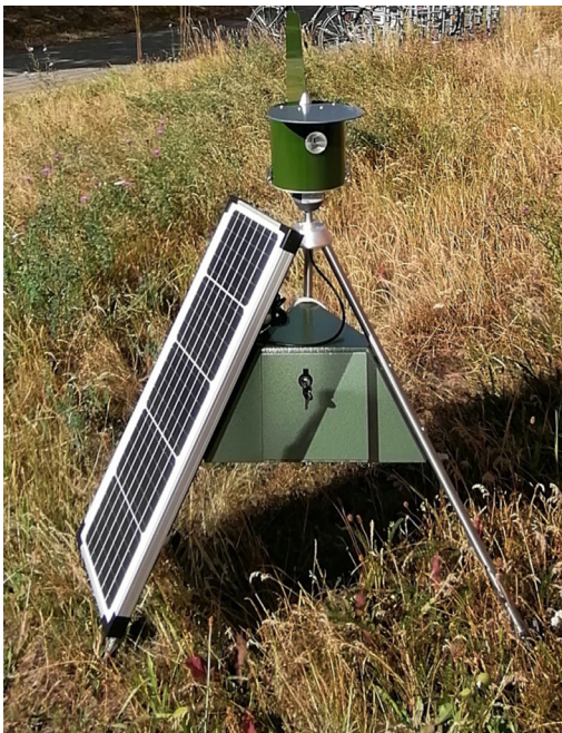
Fig. 4. Autonomous pollen sampler. Left: complete unit; right: the sample collector.
