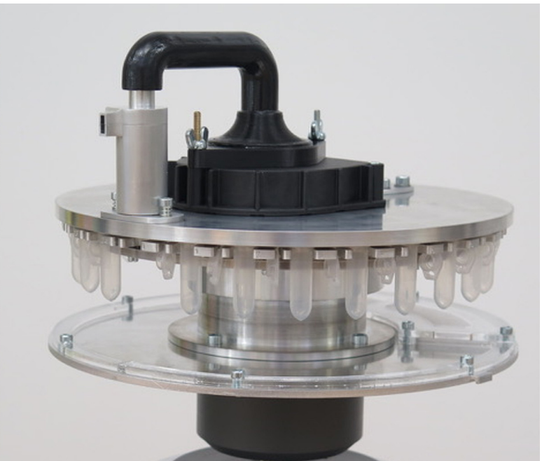
Fig. 4. Autonomous pollen sampler. Left: complete unit; right: the sample collector.
