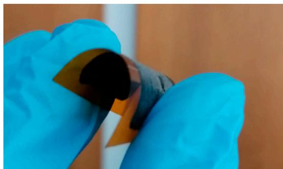
**Figure 6.** Example of the semiconducting oxide thick film on Kapton substrate.
