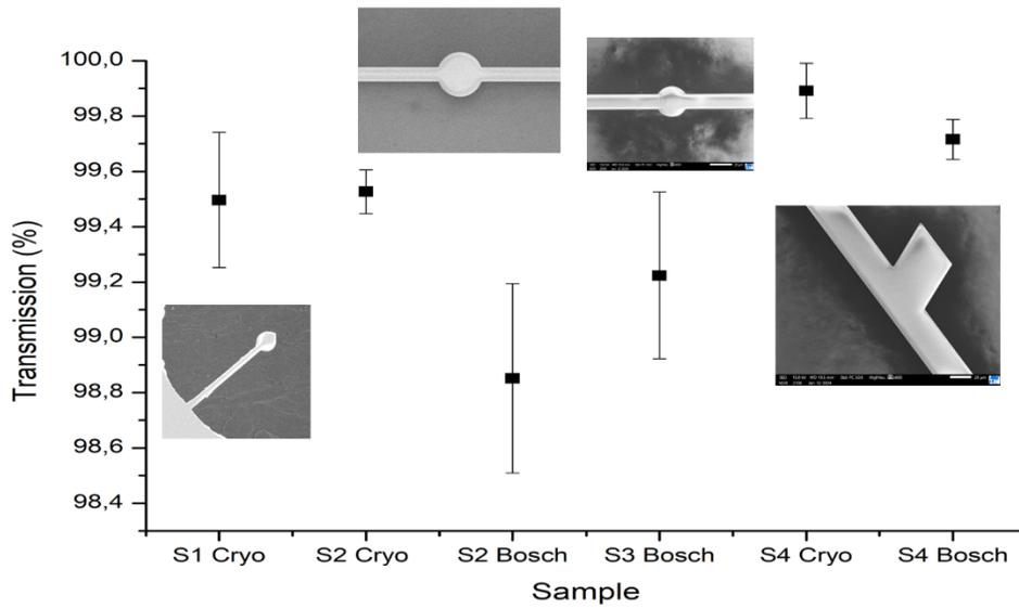
Figure 9. This graph illustrates the average measured values for fiber-to-waveguide optical transmission. Structures 1 and 2, etched by cryogenic DRIE, exhibit a transmission higher than 99.4%. Structures 2 and 3, fabricated by Bosch DRIE, demonstrate a transmission ranging between 98.8% and 99.2%. Remarkably, Structures 4, in both cryogenic and Bosch cases, showcase the highest measured transmission values.
