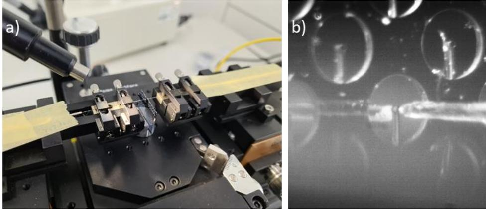
Figure 8. Picture a) provides a close-up view of the fiber-to-waveguide alignment setup. In b), the alignment of sender and receiver fibers with the integrated waveguides is achieved through a macro camera system for enhanced precision.
