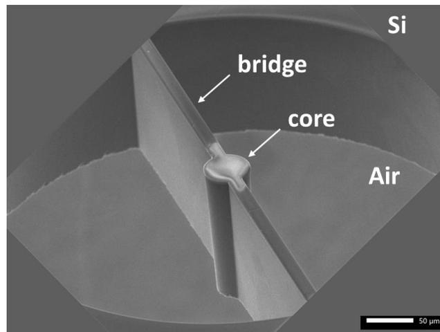
Figure 2. Scanning electron microscope image of a deep reactive ion-etched optical through-silicon waveguide. At the waveguide's top, a  $\text{SiO}_2$  layer serves as a lithographic mask. The monolithic waveguide's core is linked to the substrate through two silicon slabs. The etched trench forms an air gap, contributing to the required refractive index contrast.
