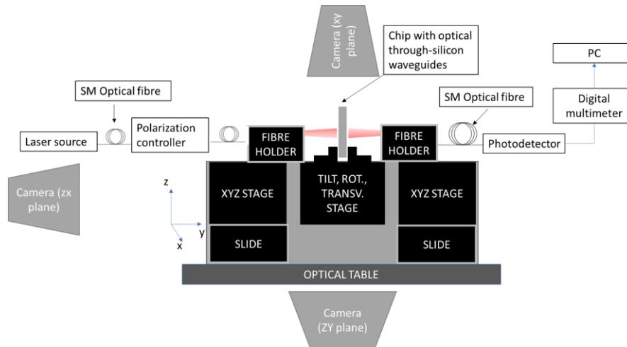
Figure 7. Schematic illustration of the optical characterization setup. The alignment of the source and receiver fibers is facilitated by an XYZ translational stage with a displacement resolution of 20 nm. In these initial experiments, two single-mode optical fibers were employed. The laser source operates at 1550 nm with a power output of 10 mW. The coupled light produces a voltage output on the receiving end. Three machine vision cameras support the manual alignment procedure.
