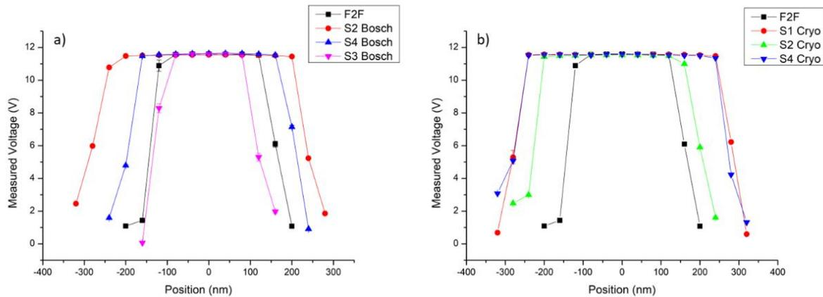
Figure 10. a) Graph depicting alignment tolerances for waveguides fabricated via the Bosch process, compared to fiber-to-fiber alignment. b) Similar representation for structures cryogenically etched. Notably, Structure 3, etched by Bosch, exhibits the lowest alignment tolerance, while Structures 2 (Bosch) and Structures 1 and 4 (cryogenic etching) demonstrate larger tolerances which are almost twice as much as the fiber-to-fiber coupling.
