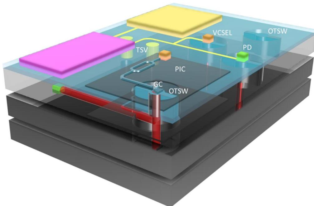
Figure 1. Graphical depiction of a three-dimensional stacked chip integration, showcasing the incorporation of diverse functions, including 3D electrical interconnects (TSV), photonic interconnects (OTSW), and various sources (VCSELs, grating couplers (GC)) and receivers (PD). A grating coupler can be designed to enable the redirection of light within a planar silicon waveguide to the vertical dimension without the need for tilting the Optical Through-Silicon Waveguide (OTSW).
