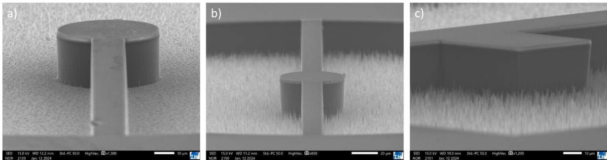
Figure 5. Scanning electron microscope images of the cryogenically etched a) Structure 1; b) Structure 2; and c) Structure 4. For etch depths up to approximately  $30 \mu\text{m}$ , the current process provides excellent morphological quality of the sidewalls with a smooth and steep profile and consistent reproducibility. At the bottom of the trenches the initial stages of black silicon/micrograss formation are visible.
