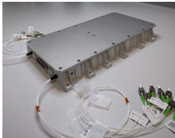
Figure 3. Fully assembled multi-core array fiber amplifier
