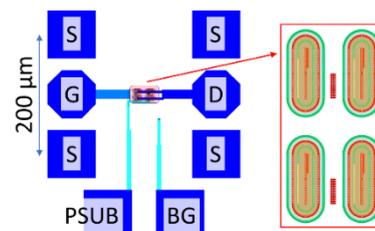
Figure 2: The parasitic influence of the pads is de-embedded to extract the properties of the PJFET.
