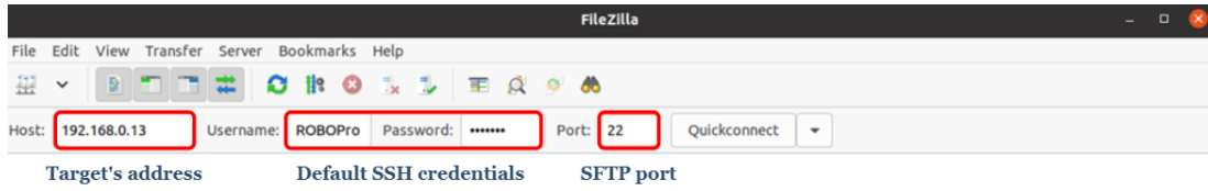
Fig. 7. Establishing an SFTP Channel with the Victim TXT Controller using Filezilla Software
