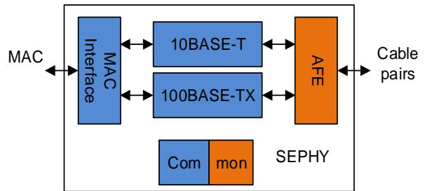
Figure 1: SEPHY block diagram
