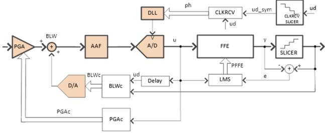
Figure 2: Block diagram of the 100BASE-TX receiver
