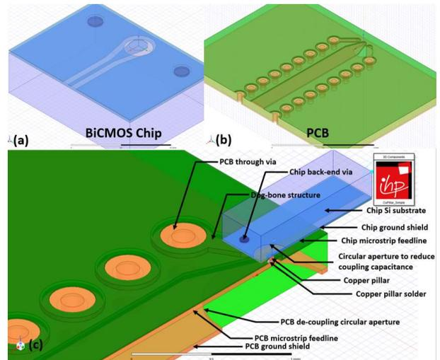
Fig. 5 The microstrip transition between the chip and the PCB. (a) is the feeding line on BiCMOS chip back-end structures, and (b) is the PCB feeding line. (c) is copper pillar interconnection assembly of the chip and the PCB.
