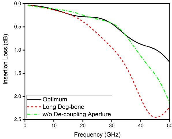
Fig. 6 The optimized insertion loss for a copper pillar microstrip transition and the influences of the key features of such a transition.
