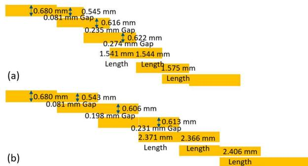
Fig. 1 The dimension of designed Bandpass filter on PCB. (a) is the geometry of the bandpass filter for transmitting band (~30 GHz), and (b) is the geometry of the bandpass filter for receiving band (~20 GHz).
