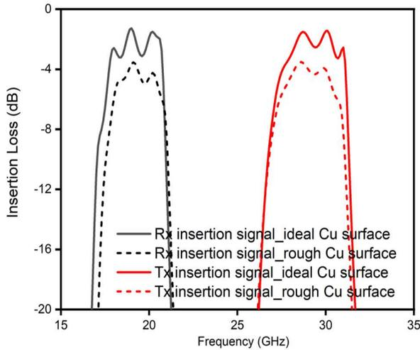
Fig. 4 The comparison of insertion losses for transceiving signals
