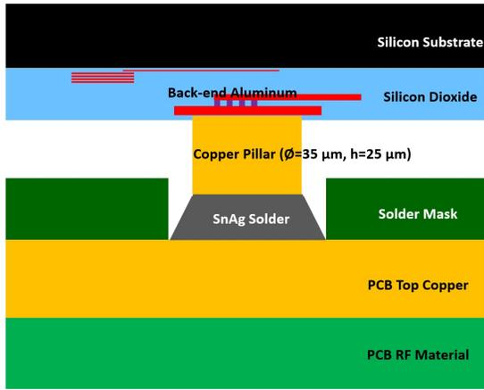
Fig. 2 The detailed cross-section view of the bump-on-pad technology using copper pillars. The interconnection is between chip and PCB.
