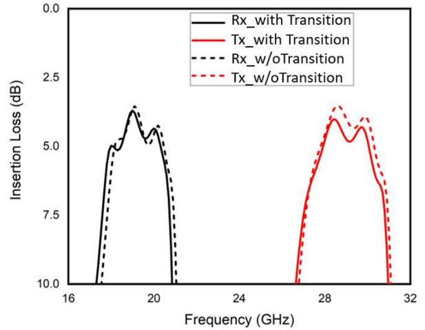
Fig. 7 The insertion losses comparison between filters with and without copper pillar microstrip transitions.
