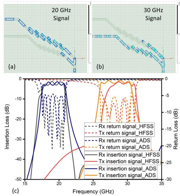
Fig. 3 The simulated performances of the diplexer on the PCB. (a) and (b) are the electric field propagating on the diplexer, corresponding to 20 GHz signal and 30 GHz signal respectively. (c) is the S parameter of the insertion and return losses of the bandpass filters.
