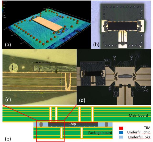
Fig. 3 An example of an assembled package with the proposed technique. (a) and (b) are the chip to package board assembly, (c) and (e) are package cross section illustrations, and (d) is the package board to main board assembly.
