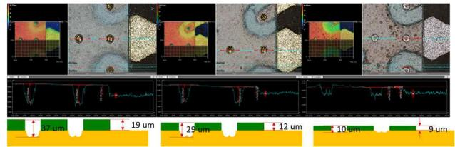
Fig. 4 The controlling of solder mask thickness.
