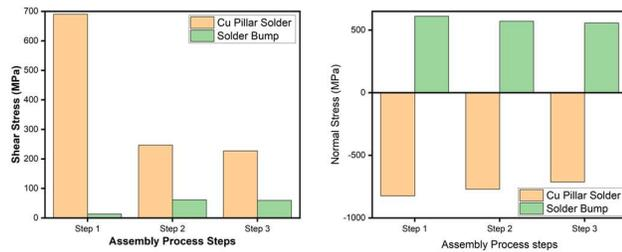
Fig. 5 The solder shear and normal stress development in the assembly process.
