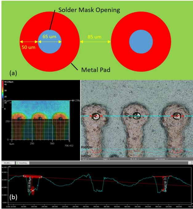
Fig. 2 The SMD pad configuration. (a) is the sketch, and (b) is the profilometry of the fabricated pads.
