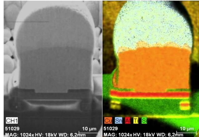
Fig. 1 A Cu-pillar example on a BiCMOS wafer.
