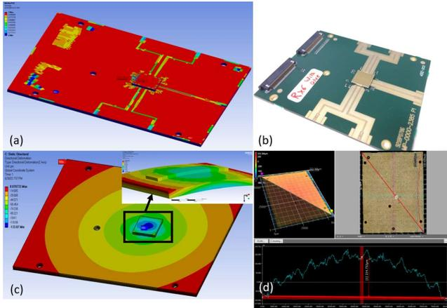
Fig. 7 The simulation and the measurement of the package warpage. (a) is the full-scale finite element model and (b) is the assembled package. (c) is the simulated package board warpage and the mother board warpage, and (d) is the package backside warpage measurement.
