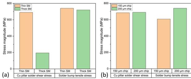
Fig. 6 the influence of the assembly process. (a) is the influence of the solder mask thickness, and (b) is the influence of the chip thickness.
