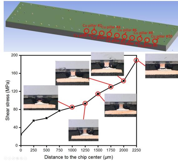
Fig. 5. The shear stresses extracted from solder joints located at different locations. The cross-sectioning of the corresponding Cu pillars are shown for comparison.
