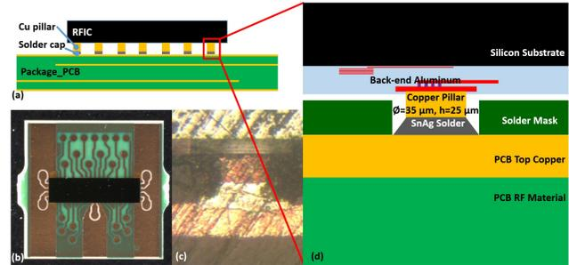
Fig. 1. The C2 flip-chip configuration. (a) is the schematic drawing of the package, (b) is the assembled package, (c) is the cross-section of the Cu pillar, and (d) is the schematic drawing of the assembled Cu pillar.
