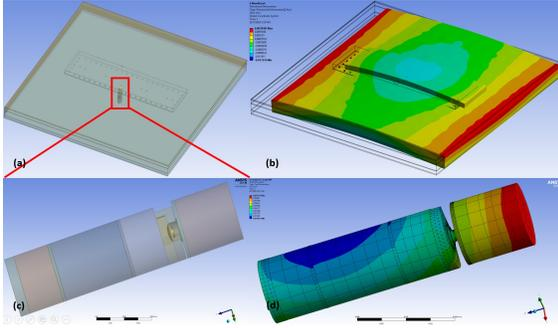
Fig. 2. The global-local modelling of the Cu pillar flip-chip. (a) and (b) are the global models of the package, (c) and (d) are the local models.
