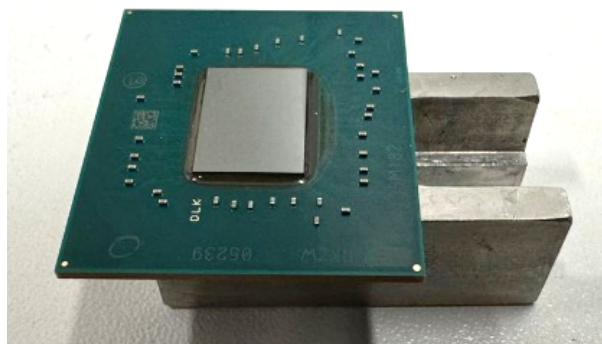
Fig. 4: Flip-Chip mounted sub 50 nm device on customized sample holder
