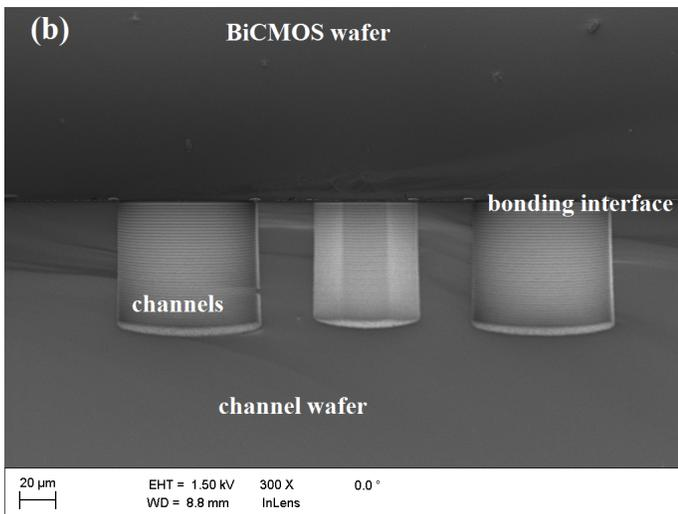
Fig. 4: Channel formation on the bonding interface (a) SEM image of the structured Si wafer bonded on the BiCMOS wafer after the backside grinding. (b) Cross-section SEM image of the channel on the bonding interface.
