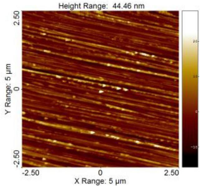
Fig. 5: AFM image of the surface after grinding
