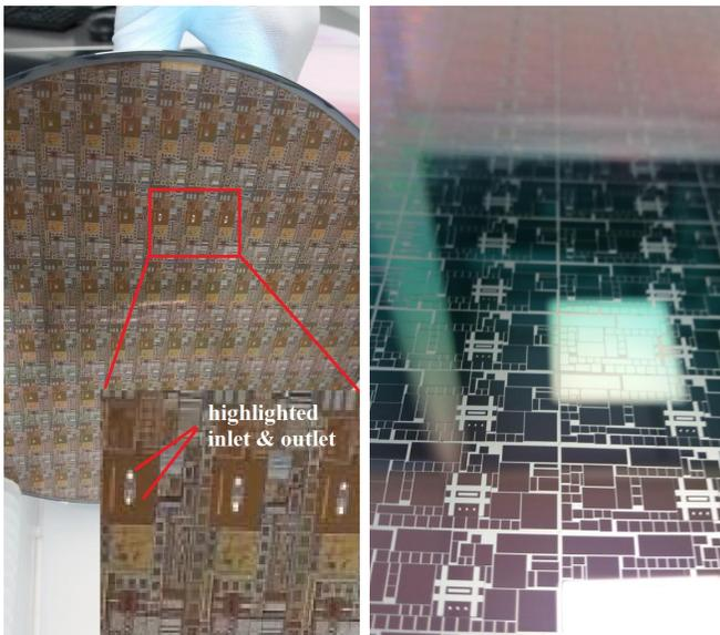
Fig. 7: Microfluidic packaging for LoC applications (the BiCMOS wafer including highlighted inlets and outlets (*left*) and the channel wafer (*right*) before integration)
