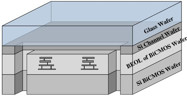
Fig. 1: 3D representation of the microfluidic channel packaging
