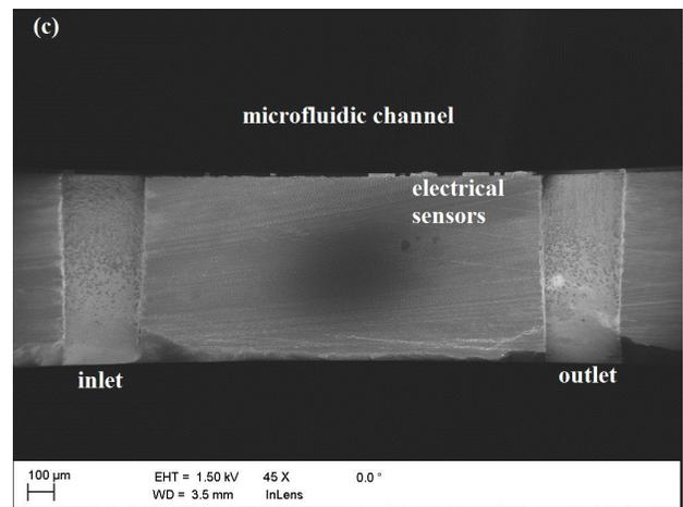
Fig. 8: Integrated microfluidic channels with sensors (a) SEM image of the sensors in the microfluidic channel (b) Top view of the channel showing the inlet of the microfluidic channel. (c) Cross-section SEM image of the system, including inlet, outlet and electrical sensors.
