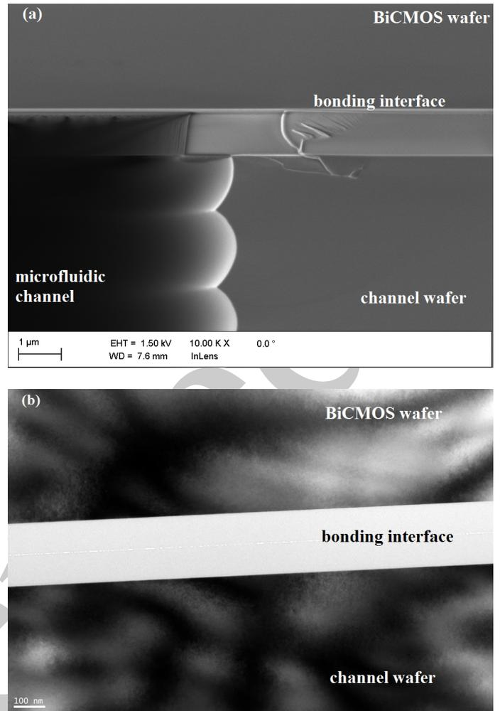
Fig. 3: Oxide-oxide bonding interface between the BiCMOS wafer and the channel wafer (a) SEM image of the interface (b) TEM image of the interface
