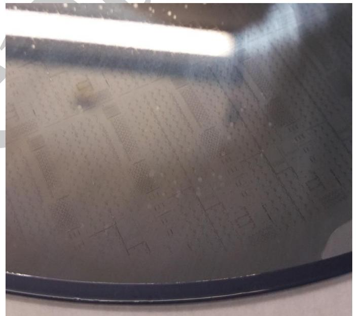
Fig. 6: 3-wafer-stack after glass wafer bonding, channel structures are visible on image.
