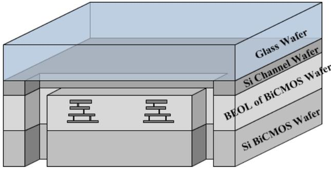
**Figure 1** 3D representation of the microfluidic channel packaging.
