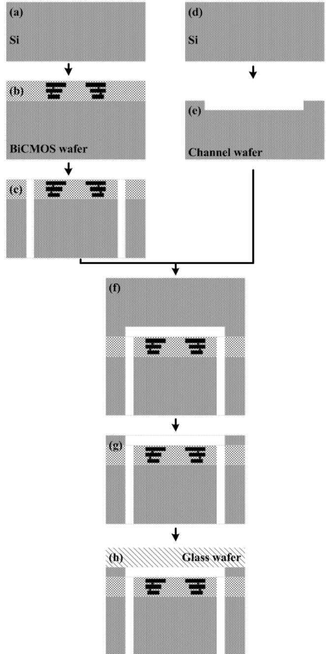
**Figure 2** Schematic representation of the microfluidic packaging processes steps. On a Si wafer (a), active circuitry (b) and microfluidic inlets (c) are opened and this wafer bonded (f) together with a channel wafer (e) built on a bare Si wafer (d). After the grinding (g) and adhesive bonding steps (h), transparent microfluidic channels are encapsulated.
