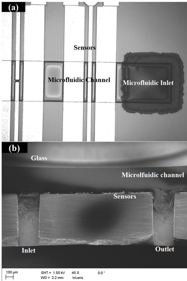
**Figure 5** Demonstrated LoC systems (a) top view of microfluidic chip including microfluidic inlet and sensors (b) cross-section image of microfluidic LoC system.
