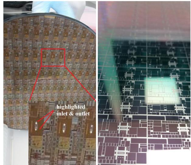
**Figure 4** Microfluidic packaging for LoC applications (the BiCMOS wafer including highlighted inlets and outlets (left) and the channel wafer (right) before integration)
