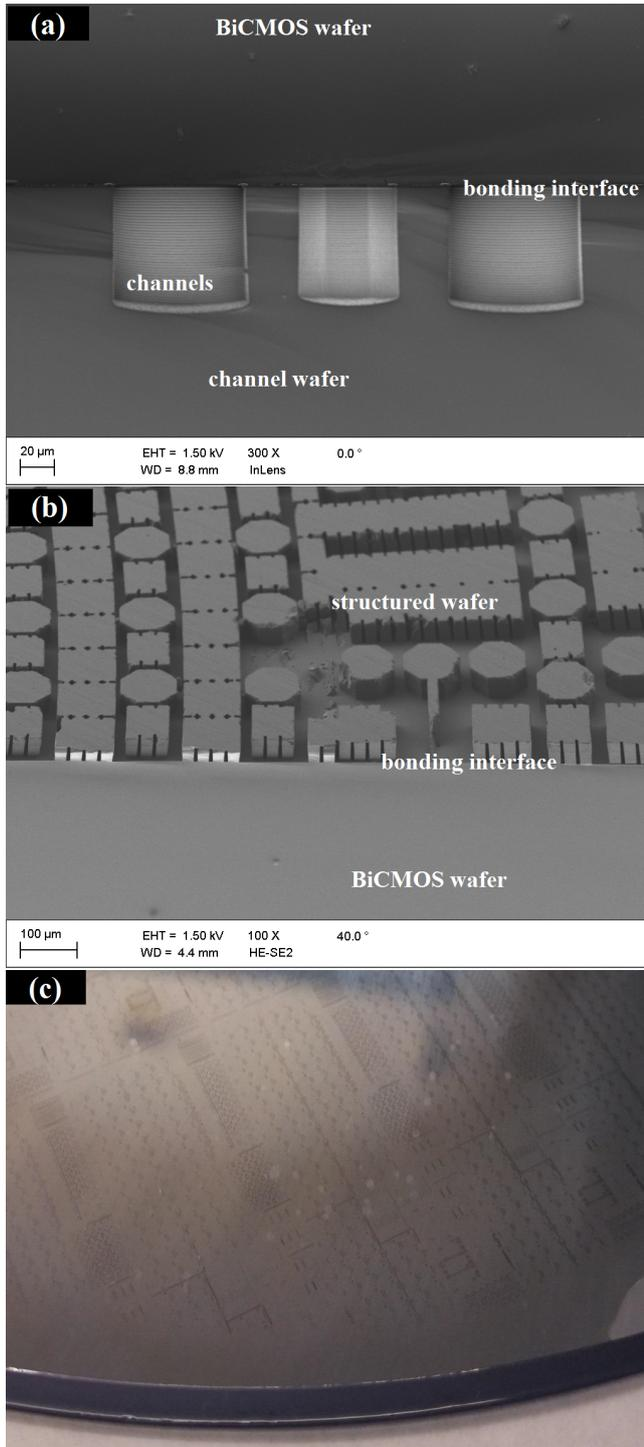
**Figure 3** Demonstrated process flow steps (a) Channels after fusion bonding (b) Bonded wafer after backside grinding for exposing the channels (c) 3-wafer stack after glass bonding.
