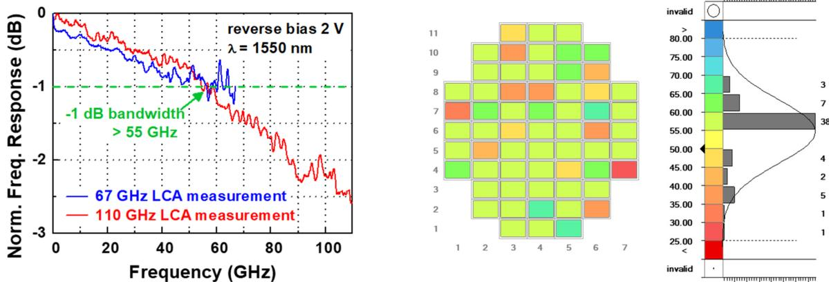
Fig. 4.: Normalized frequency responses (left, [2]) of one chip (diode "Ge-300") measured with Keysight 67 GHz LCA and 110 GHz LCA, all at 1550 nm. Wafermap and histogram (right, [2]) of 1-dB OE bandwidths of "Ge-300" PD at -2 V (in GHz), measured on 62 wafer sites, 1550 nm wavelength.
