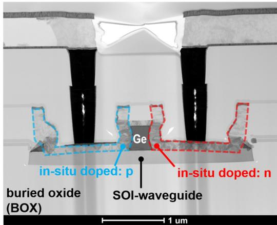
Fig. 1: STEM cross section of photodiode "Ge-300" (left) and frequency responses (right) measured with 110 GHz LCA at 1550 nm wavelength (four chips from the same wafer).
