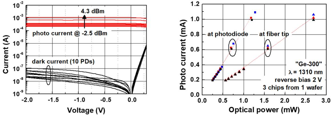
Fig. 3: Dark- (10 PDs) and photo-currents (one PD) at 1310 nm (left); Photo-current vs. optical power for the estimation of external (at fiber tip) and internal (at PD) responsivities (right). All measurements: PDs "Ge-300" on chips from the same wafer.
