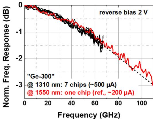
Fig. 2: Frequency responses (left) measured with 67 GHz LCA at 1310 nm (7 diodes from the same wafer from the follow-up lot) and, for direct comparison, 110 GHz LCA measurements at 1550 nm (red curve, measured on wafer from first lot). Capacitance-voltage characteristics from diodes of 2nd lot compared to those from prior photodiodes (right).
