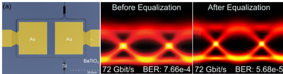
Fig. 2: (a) SEM image of ferroelectric plasmonic Mach-Zehnder modulator; (b) 72 Gb/s eye diagram and measured BER before equalization; (c) 72 Gb/s eye diagram and measured BER after equalization.
