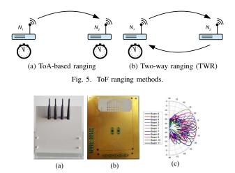
Fig. 6. Analog front-ends (AFEs): a) Sub-6 GHz dipole antenna array, b) 60 GHz antenna array, and c) beams associated with the 60 GHz antenna array.
