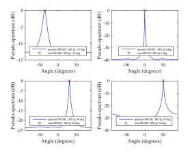
Fig. 7. AoA estimation of the pilot tone impinging the antenna array at the angles -35, 0, 30 and 50 degrees.
