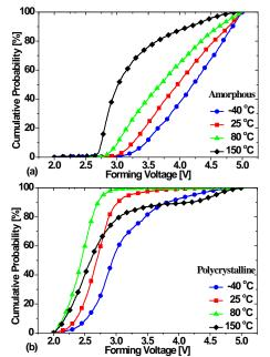
Fig.5: Forming voltage cumulative probabilities at the selected temperature values in A-arrays (a) and P-arrays (b).
