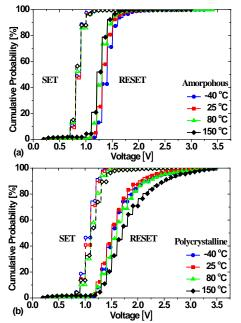
Fig.7: Reset and set voltage cumulative probabilities at the selected temperature, respectively, in A-arrays (a) and P-arrays (b).
