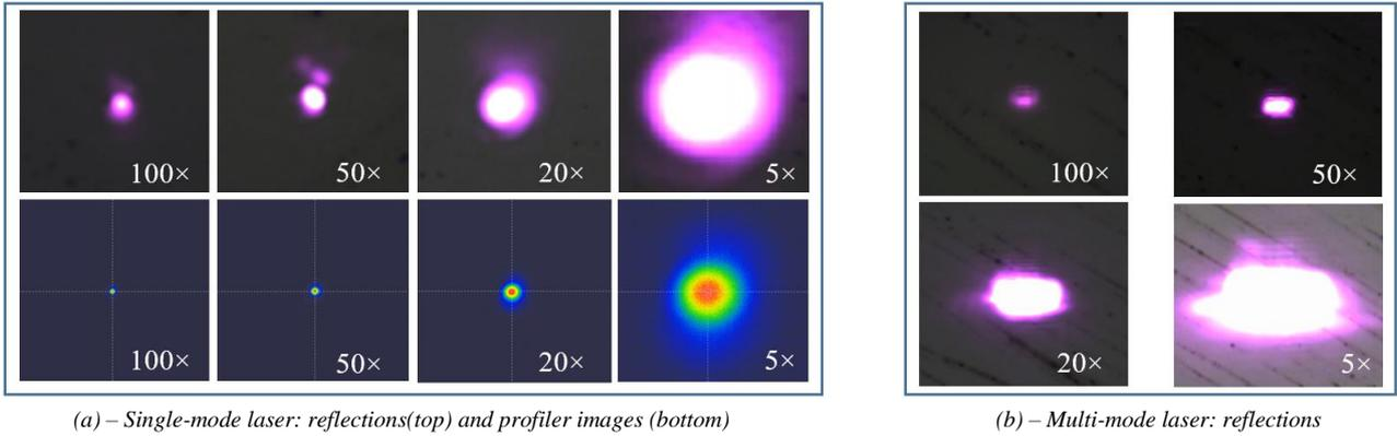
**Fig. 4.** Reflections of the laser beam spots from silicone surface for the red single-mode and the red multi-mode laser as well as images captured using a laser beam profiler for the red single-mode laser.
