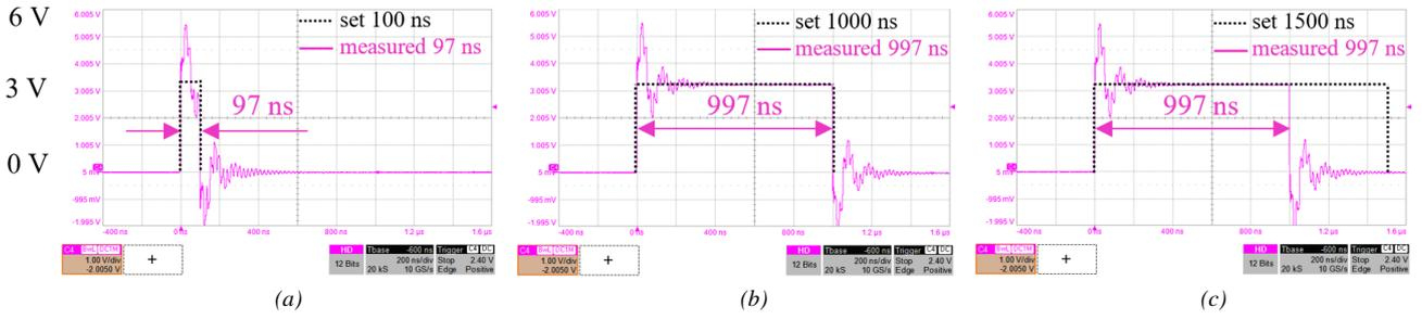
**Fig. 3.** Measured oscilloscope waveform of the “laser beam pulse duration” signal generated at the output of the VC glitcher. The signal durations were set in the Inspector FI software as follows: (a) – 100 ns; (b) – 1000 ns; (c) – 1500 ns.
