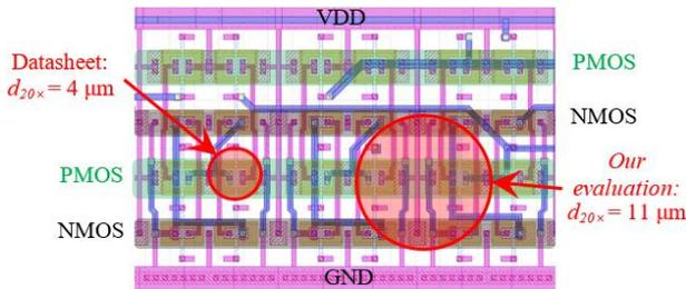
Fig. 1. Part of the attacked cell and comparison of laser beam spot sizes taken from the datasheet and experimentally measured.
