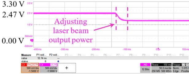
Fig. 2. Measured oscilloscope waveform of the “laser beam output power” signal generated at the output of the VC glitcher. The voltage level adjusts to 1.83 V for the first laser shot, i.e. 50 % “power”.
