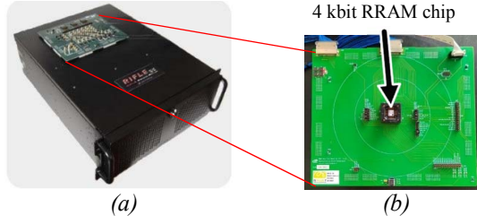
Fig. 7. Operating device for a 4 kbit RRAM chip: (a) – Active Technologies RIFLE SE; (b) – a PCB with a socket for a 4 kbit RRAM chip.
