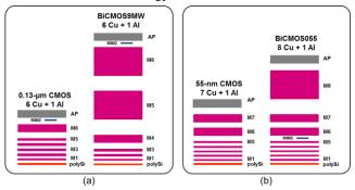
Fig. 3. Exemples of BEOL modifications between the digital CMOS and derived BiCMOS at STMicroelectronics in 0.13  $\mu$ m (a) and 55 nm (b).
