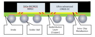
Fig. 8. Proposal for a System in Package (SiP) with a BiCMOS MMIC and an IC from a very advanced CMOS node.
