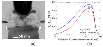
Fig. 2. From [10] a) TEM cross section of a HS HBT in BiCMOS055 [11]. (b) Corresponding  $f_{T}$  and  $f_{MAX}$  vs. collector current density.
