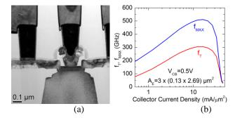
Fig. 5. (a) TEM cross section of an HBT with elevated extrinsic base and 130 nm emitter width (from [26]), (b) Corresponding  $f_{\rm T}$  and  $f_{\rm MAX}$  vs. collector current density.
