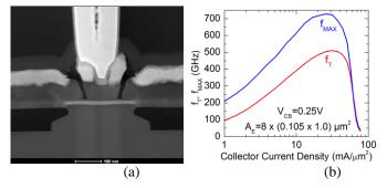
Fig. 6. (a) TEM cross section of an HBT with elevated extrinsic base and 105 nm emitter width (from [17]). (b) Corresponding  $f_{\rm T}$  and  $f_{\rm MAX}$  vs. collector current density.
