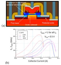
Fig. 7. a) TCAD cross-section of the EXBIC architecture. b)  $f_{\rm T} \& f_{\rm MAX}$  from B55X (cf. IV.C.2) tentative HICUM model based on TCAD simulations.
