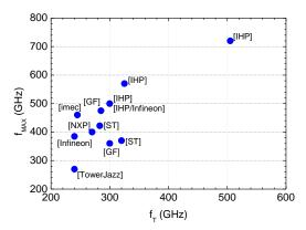
Fig. 1. Peak  $f_{\rm T}$  and  $f_{\rm MAX}$  values of high-speed SiGe HBT technologies (references are available in [10]).
