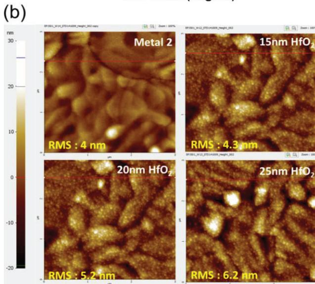
**Figure 2** (a) XRD peaks for AVD  $\text{HfO}_2$  films deposited at  $400^\circ\text{C}$  and (b) AFM topography measured on metal 2 (i.e., AVD TiN BEs), 15 nm AVD  $\text{HfO}_2$  films, 20 nm AVD  $\text{HfO}_2$  films, and 25 nm  $\text{HfO}_2$  films. This figure also shows their root mean square (RMS) properties.
