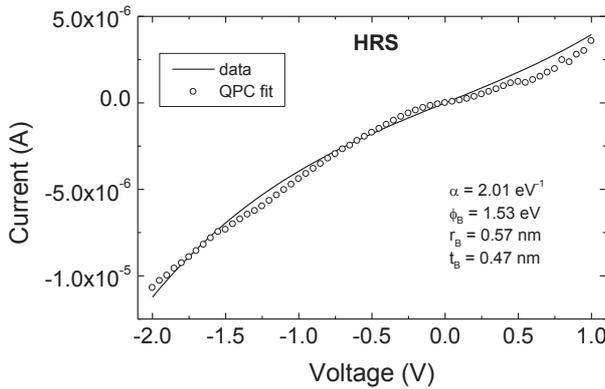
**Figure 4** Experimental and theoretical I-V characteristics for the HRS. The QPC model (Eq. (1)) was used for the theoretical curve.
