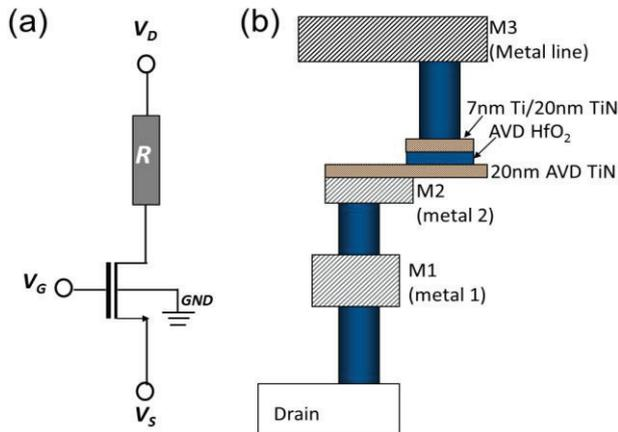
**Figure 1** (a) Equivalent circuits of fabricated  $\text{HfO}_2$ -based 1T1R RRAM cells and (b) schematic of RRAM devices with AVD TiN bottom and AVD  $\text{HfO}_2$  films on drain.
