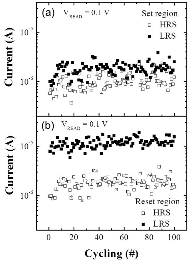
**Figure 4** The dc cycling characteristics of 100 times in (a) RESET and (b) SET voltage regions at  $V_{\text{READ}} = 0.1\text{V}$  for 15 nm AVD  $\text{HfO}_2$  1T1R RRAM cells.
