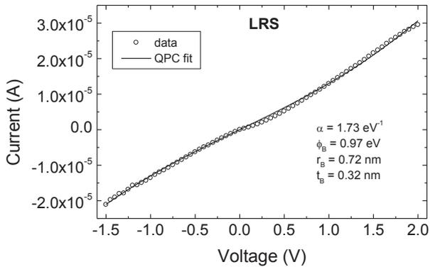
**Figure 5** Experimental and theoretical I-V characteristics for the LRS. The QPC model (Eq. (1)) was used for the theoretical curve.
