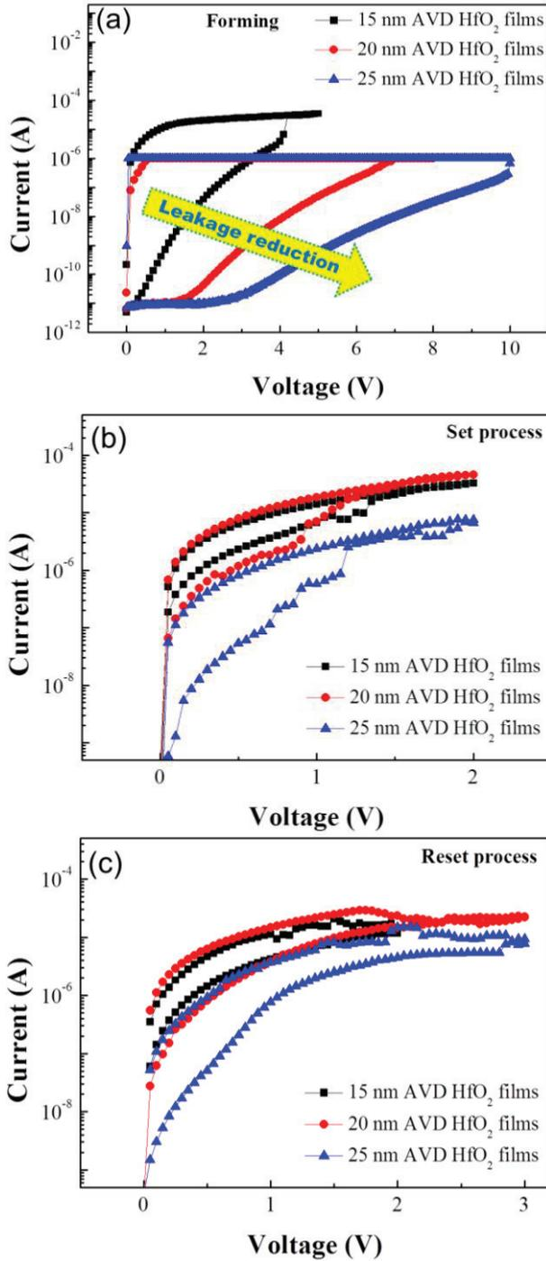
**Figure 3** (a) Forming, (b) SET and (c) RESET characteristics for AVD HfO<sub>2</sub> based 1T1R RRAM with different thickness of 15 nm, 20 nm, and 25 nm HfO<sub>2</sub> films.
